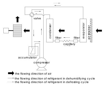
Other main working components are: high efficient compressor, accumulator, magnetic flow control valve, evaporator coil, condenser coil, capillary tube, centrifugal fan, temperature sensor, humidity sensor and electrical wiring.
